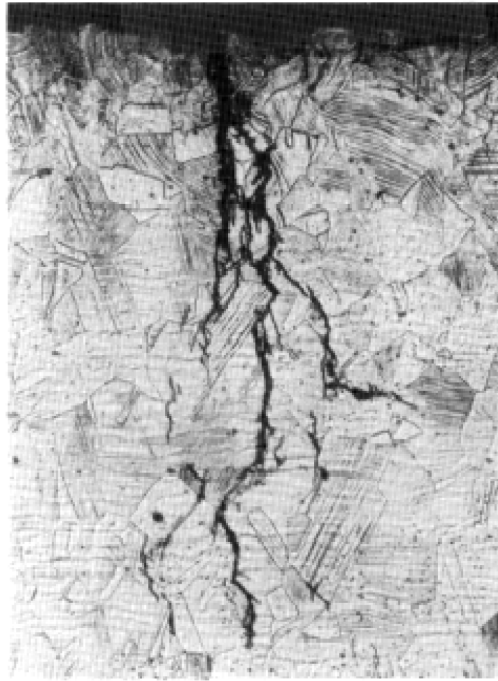
Figure 2-31. Micrograph of a Cross-Section Through a Stress-Corrosion Crack
