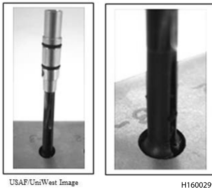
Figure 4-36. Checking Probe Fit
