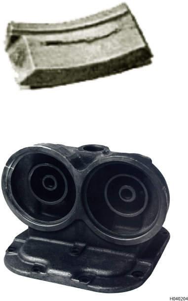
Figure 3-59. Magnetic Particle Indications of Defects in Castings
