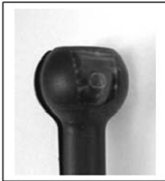
Figure 4-37. Examples of Acceptably Taped Bolt Hole Probes
